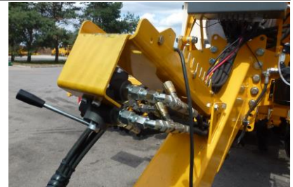
Figure: 2: Flow directing valve (marker - locking latch)
