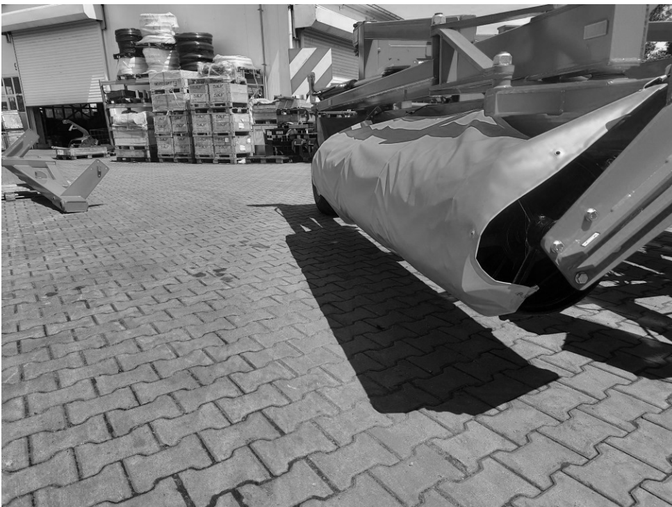
Photo no. 2. Tarpaulin cover for the external elements of the machine - left side of the shaft.
