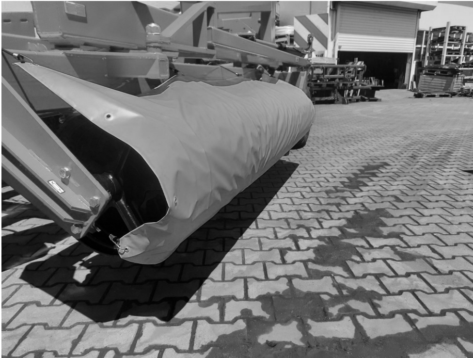
Photo no. 1. Tarpaulin cover for the external elements of the machine - right side of the shaft.
