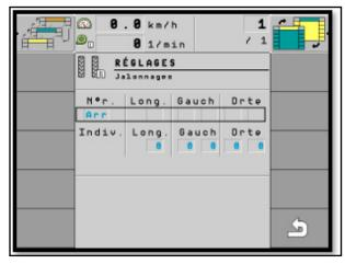
4 - Use the knob to scroll in this screen and press the knob to validate.
