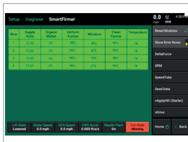
The screenshot shows the 'SmartFirmer' diagnostic screen. At the top, it displays 'Setup > Diagnose > SmartFirmer'. Below this is a table with columns: Row, Supply Volts, Organic Matter, Uniform Furrow, Moisture, Clean Furrow, and Temperature. The table contains four rows of data:
