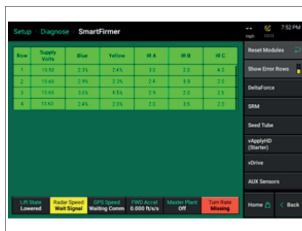
The screenshot shows the 'SmartFirmer' diagnostic screen. At the top, it displays 'Setup > Diagnose > SmartFirmer'. Below this is a table with columns: Row, Supply Volts, Blue, Yellow, IR A, IR B, and IR C. The table contains four rows of data:
