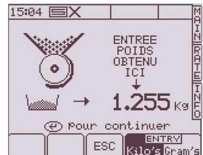
5. Press ENTER again and the console recalculates and displays the new calibration factor in kg/rev, the error %, and the maximum permitted forward speed calculated according to the application rate set for the product (Fig. 15).
