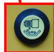
***Fig. 17: button to activate the seeding rate test***
