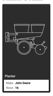
The Planter Details screen allows for configuration, saving, and loading of different planter profiles.
