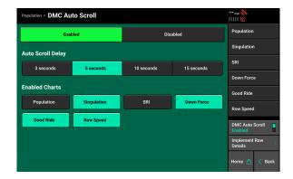
**Note:** As of software version **2024.1.1**, there is a visual bug when accessing the Row Details screen by using the Implement Row Details button on the DMC Auto Scroll screen. Use the Implement Row Details button on the Metric screen instead to access the Row Details Screen.
