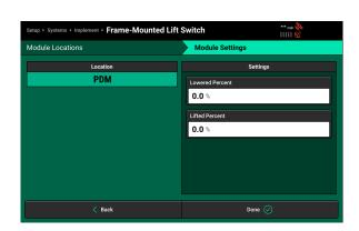
SmartFirmer — Configures one or multiple SmartFirmers on the implement. After selecting all module row locations, use the Module Settings screen to view/change active sensors. See the SmartFirmer Operator's Guide for more details on using SmartFirmers.
