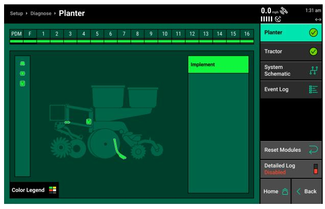
Press Implement on the center screen graphic. Press the desired module to view a chart of the diagnostic information available for that module(s).
