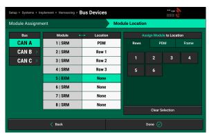
Press the number 3 or 4 to assign module 5 | BXM to either of those locations. A BXM must be assigned to a row (or tower in Air Seeder mode) even if it is physically mounted to the frame. Use the closest row or tower to the physical location of the BXM for identification purposes.
