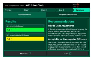
Press Equipment Measurements to view a detailed comparison of the measurements performed in Equipment setup and the measurements calculated during GPS Offset Check.
