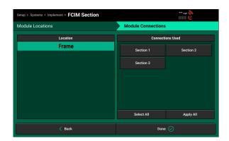
After selecting active connections, use the Module Settings screen to assign the rows that are controlled by each connection. Press on each Frame Section under Location to select it, then manually select which rows are controlled by that connection from the Assign Rows table.
