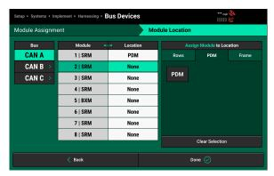
Press Rows under Assign Module to Location, then press the number 1 to assign module 2 | SRM location to Row 1. Continue assigning the correct row locations to Modules 3\4| SRM.
