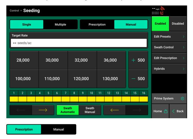
Press Prescription at the top of the control screen to switch from manual to prescription control. The system will now control to the assigned prescription file.
