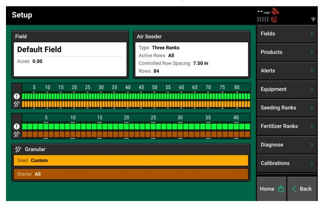
When in Air Seeder mode with Seeding and Fertilizer ranks selected in Equipment, Systems will be replaced by two options that read Seeding Ranks and Fertilizer Ranks. Use the following guidelines when configuring systems and harnessing for seeding and fertilizer ranks.
