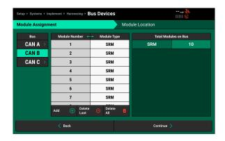
Press Delete Last to remove the last bus device in sequence from the selected CAN network. Press Delete All to remove all bus devices from the selected CAN network.
