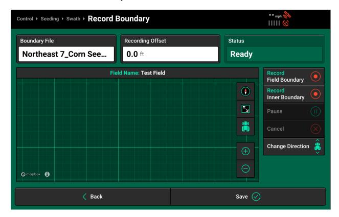
Press Boundary File to select the file name for the new boundary, or press Create New Boundary on the pop-up to enter the desired boundary name.
