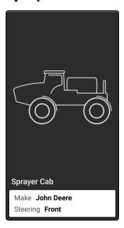
The Sprayer Cab Details screen allows for configuration, saving, and loading of different cab profiles.
