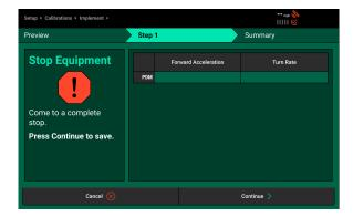
Drive forward and turn to confirm that the gyro is reading both acceleration and turn rate. Both values will be displayed in the on-screen chart.
