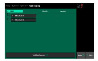
Press the dropdown arrow next to a CAN network to view the detailed schematic for that network. Scroll down on the table to view all modules or select another network.
