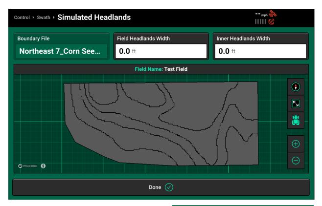
Press Field or Inner Headlands Width and enter the desired value for the selected headland type using the pop-up.
