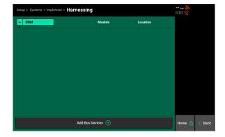
Ensure CAN A is highlighted in the Bus list. Press Add + in the center screen table.
