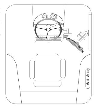
The DBM may be located in any convenient area of the cab. Ensure the DBM will remain stationary when operating the tractor. Connect one end of the provided Ethernet cable into either port on the DBM and the other end into the display port. If using two displays, connect the second display with the provided Ethernet cable to the other open port on the DBM.
