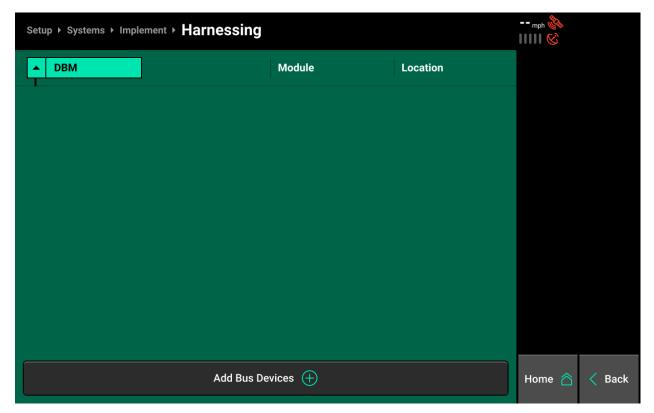
Press Add Bus Devices to open the Bus Devices screen. This screen allows the user to set up all other bus devices and CAN networks. No systems will function until bus devices and CAN networks have been set up on the 20|20 in the same configuration that those devices and networks are laid out physically on the implement.
