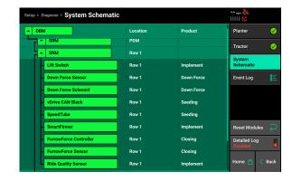
Use the black brackets leading from the DBM to the different bus devices to verify the physical layout of CAN harnessing.
