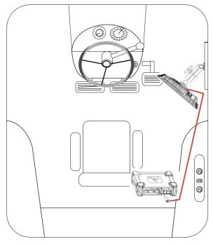
Connect the 725150 Power Harness into the 4-pin Deutsch Connector on the DBM and then to the power source in the tractor cab. A three pin round convenience port connector is provided to plug directly into a standard convenience port. Various adapters are available to connect to different power sources.
