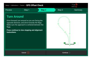
Stop when the flags/markers are aligned with the application points.
