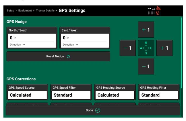
Use the +1/-1 buttons nudge GPS when experiencing signal drift on lower accuracy systems. Use the +1 buttons to nudge GPS North or East 1 inch, and the -1 buttons to nudge GPS South or West 1 inch Use the Reset Nudge button to erase all nudge settings. Press the dimensions below North/South and East/West to manually enter a value using the pop-up keyboard.
