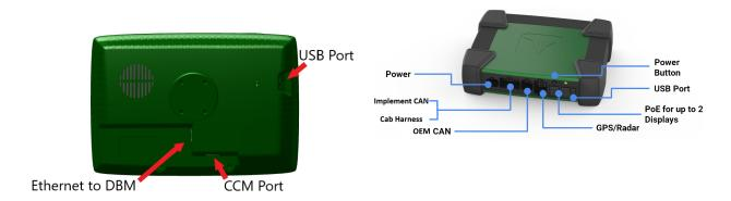
The Power over Ethernet [PoE] ports require a Shielded Twisted Pair [STP] Ethernet Cable to connect to a display. If only one display is being used, use either port. Both ports will be used if connecting to two displays or one display and a FieldView Module [FVM]. The display(s) or FVM may be plugged in to either port.
