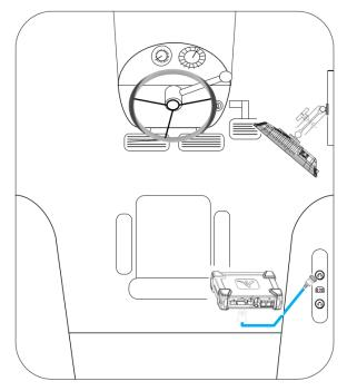
Connect an Implement CAN Harness into the 12-pin Deutsch Connector on the DBM. Route the remaining length of the cable through the cab harness port in the back window. There will be two CAN connections on the harness, CAN A (black connector) and CAN B (brown connector). If a PDM is installed on the implement, CAN A must be used and routed to the PDM.
