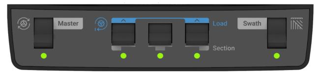
The switch on the left hand side is the Master Plant switch. For all control products to function the Master Plant switch must be in the up position. If it is in the down position, all control products will immediately be disabled.
