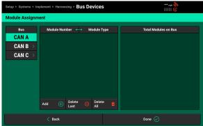
Select the desired CAN network from the Bus list on the left side of the screen, then press Add + to add bus devices. Different bus devices will be available depending on equipment setup.
