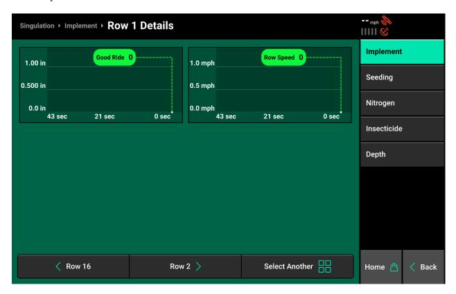
The Row Details screen allows the user to view all available information for the selected row in order to maximize implement performance. Select a different system using the navigation menu on the right side of the screen. Different options will be available based on configured systems.
