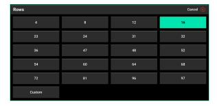
Press the number under Row Spacing to select a preset spacing, or to enter a custom number. Row pacing refers to the physical spacing between all rows on the implement.
