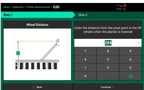
Follow the on screen instructions to physically measure the indicated dimension of the implement, and input the measurements step-by-step into the 20|20. Press Done after all measurements are input.
