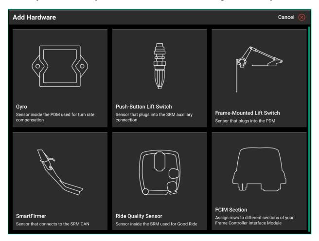
Gyro (PDM systems only) — Configures the gyroscopic sensor. Assign the gyro location to the PDM, then use the Module Settings screen to view the Gyro Zero Offset, change PDM mount location/orientation, or to disable the Gyro.
