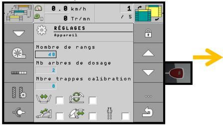
– Select the options of the machine, with the scroll wheel, and press button 8
