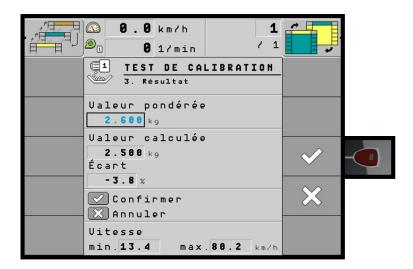
19 – The factor of calibration can be modified after each tests according the result gotten. The procedure, needs to be repeated until the weight is close to the theoretical one (+ or -5 % error allowed) Speeds indicated are the distribution's limits of the working range.
