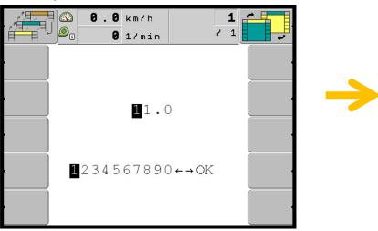
11 – Put the quantity at 150 Kg/ha (if it is the first use) with the scroll wheel and validate pressing on
