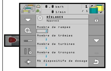
**26** – Set the width of the tool, with the scroll wheel for section 1 and 2 (button 9 to change) and restart the monitor.
