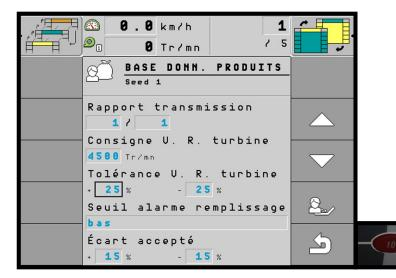
13 – Check the tolerance at + or – 25%.
