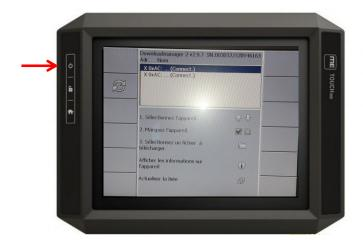
**4** – Select the setup of seeder expected and press the line expected.
