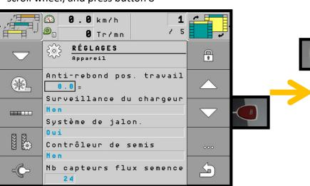
Select the options of the machine, with the sroll wheel, and press button 8
