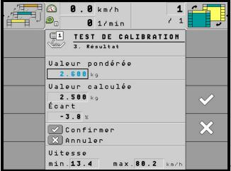
**17** – Enter the weight with the scroll wheel to validate on
