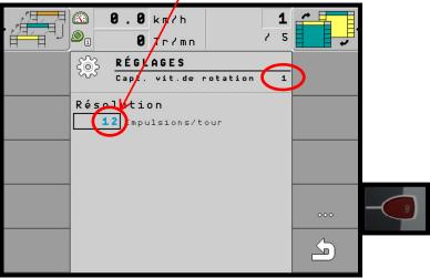
**22** – Press the button 9 to have the sensor 5 Check the value of 2 impulsions.
