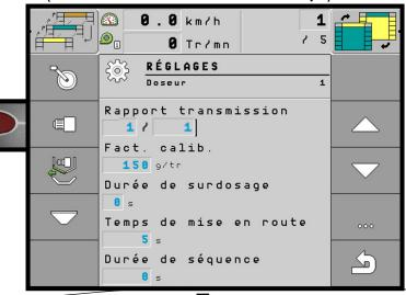
**20** – Check the value of the motor and the ratio, or modify, and press button 1
