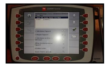
**2** – Press the scroll wheel top right or touch B and switch on the monitor; the screen appears after a few seconds.
