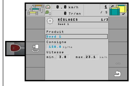
**6** – Enter the quantity with the scroll wheel and validate pressing on the scroll wheel
