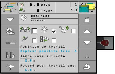
– Check the option of the machine with the scroll wheel and press button 8
