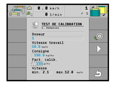
**13** – Put FACT. CALI at **150** g/tr with the scroll wheel to validate pressing on
