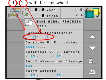
**12** – Come with the scroll wheel to modify the speed setup at 4500 tr/mn.
