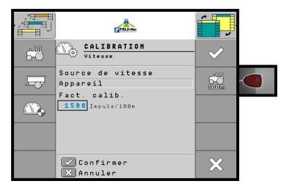
**12** – Press the button 8 and drive100 m with the tractor
