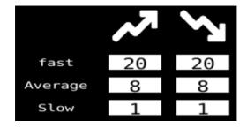
These settings correspond to the acceleration and deceleration of the engine depending on the deviation from the regulation.
