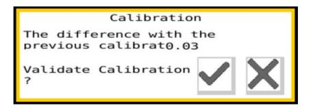
The error rate is displayed, VALIDATE. If the error is greater than 5%, restart a calibration.
